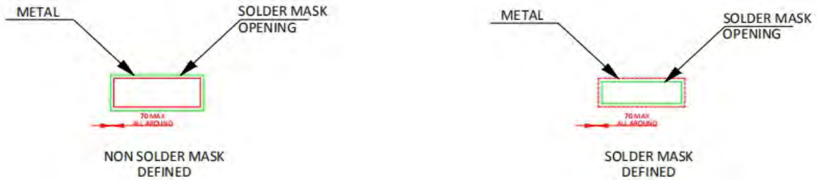
Figure 9.3 SOW8 Package Board Layout Example
